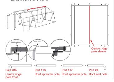
• Install the side ridge poles x2. Select the frame (parts #3, #18, #17 and #4) for the side ridge poles and insert through the centre ridge pole sleeve on the roof of the tent, ensuring the front pole #3 is correctly fitted through the webbing loop and pole sock and the rear pole #4 is fitted through the webbing strap attached to the tent.
