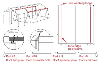
WARNING - Do not force poles through the sleeves as this may damage the sleeve. Check to ensure the pole does not snag when sliding it through the sleeve.
