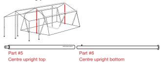
WARNING - Do not push the poles up too high as this may cause undue stress and damage to the fabric.
